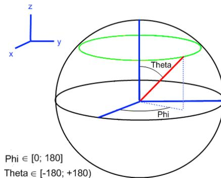
**Fig. 2** Definition of spherical coordinates for measured data
