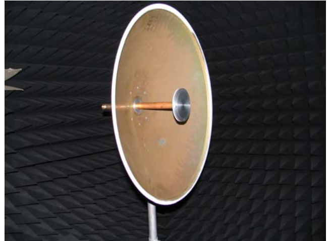
Fig. 7 Antenna assembly measured in anechoic chamber
