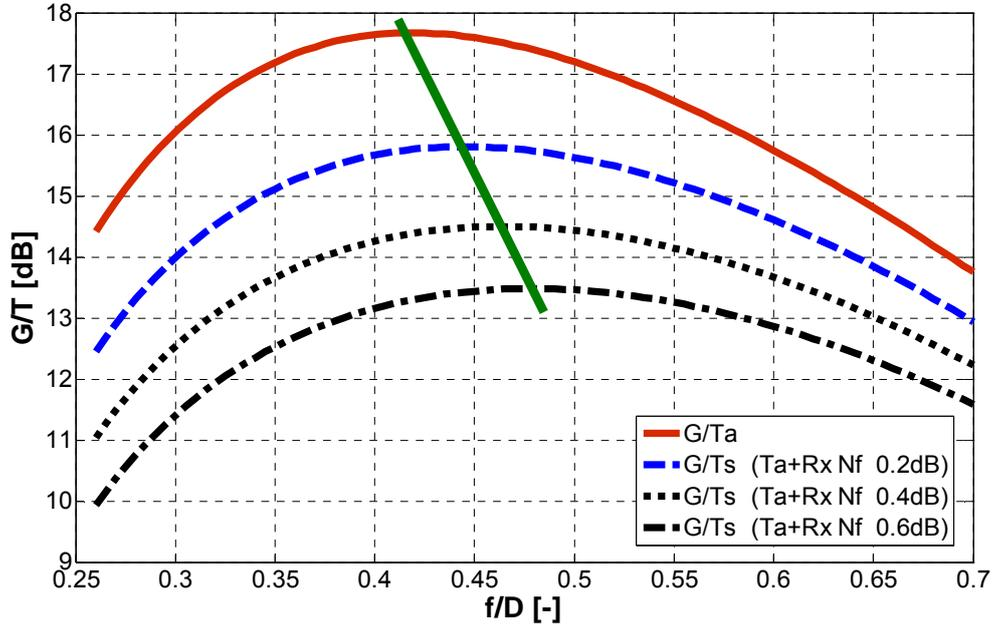
Fig. 9 - Antenna and System  $G/T$  ratio
