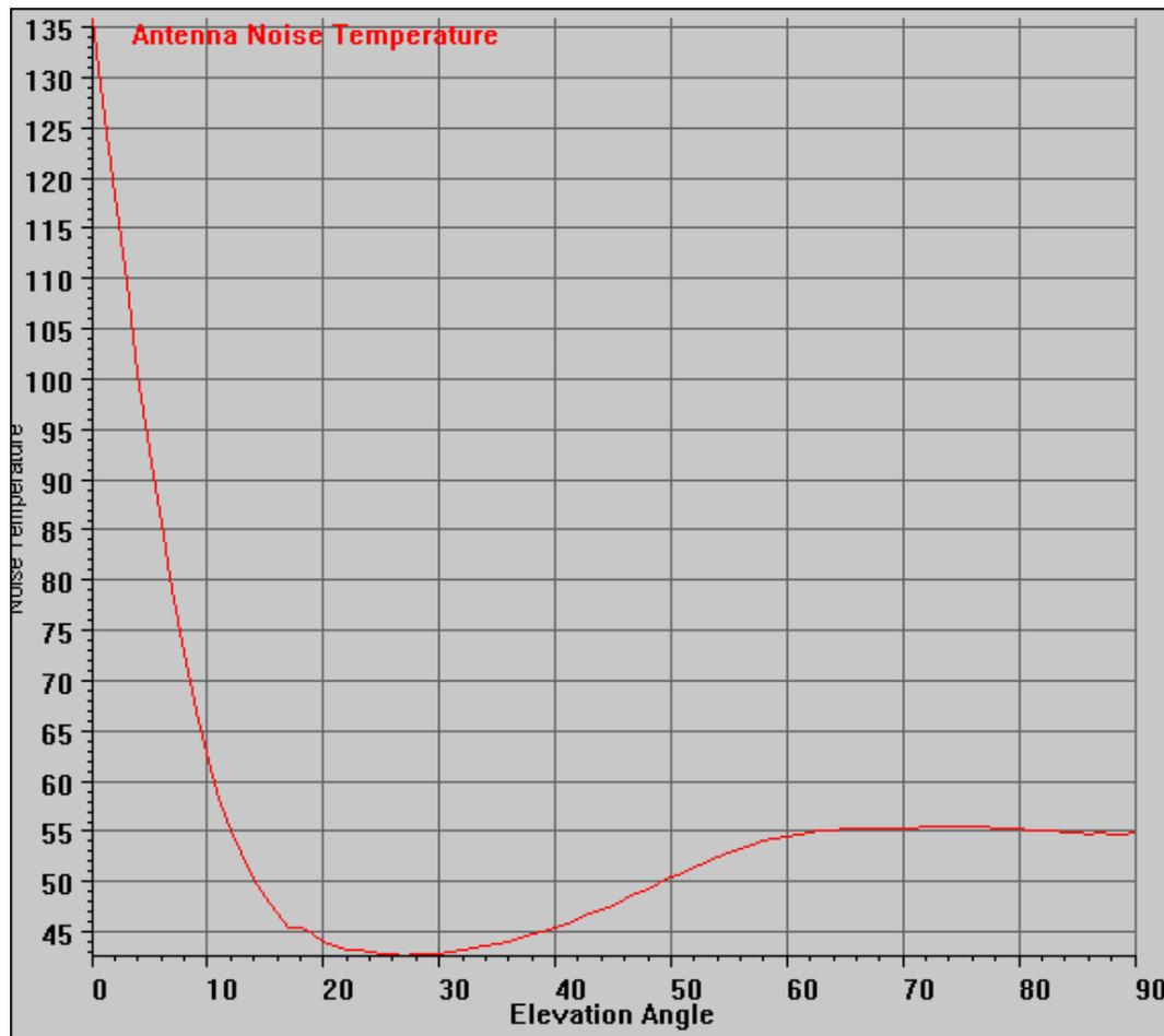
**Fig. 7** - Dependence of antenna noise temperature on elevation angle for a dish with f/D ratio 0.65. Note accrual of antenna noise temperature for higher elevation angles, above 50 degrees, due to antenna spillover.
