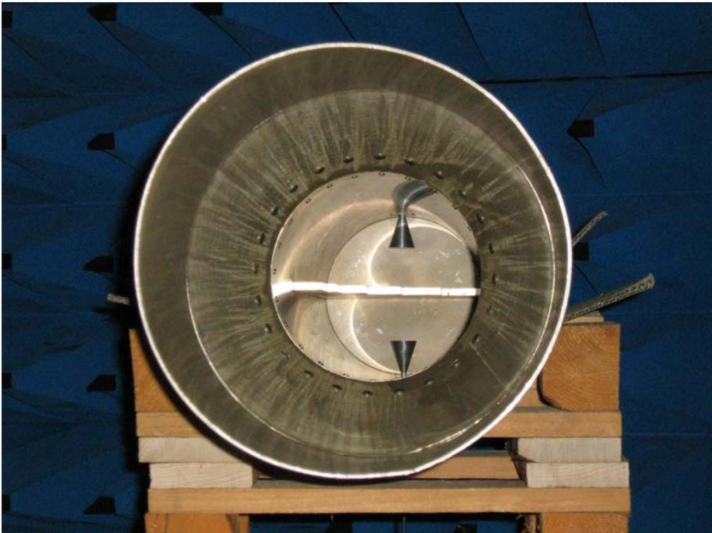
**Fig. 3b** - Real dual-mode feed, front view
