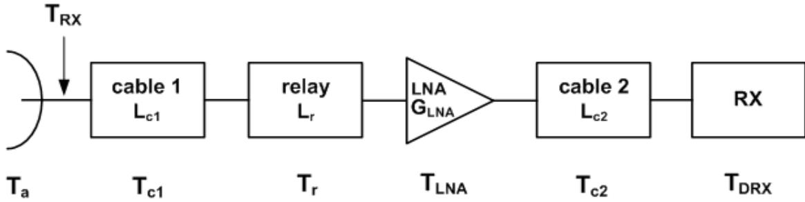
**Fig. 2** - Block diagram for noise temperature calculation of a typical system
