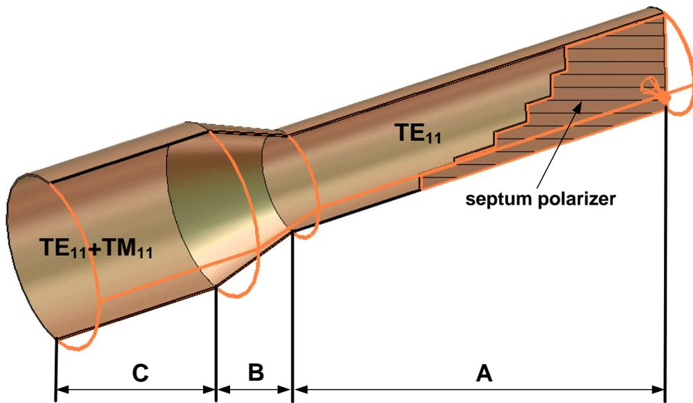
**Fig. 3a** - Dual-mode feed, CST MWS model
