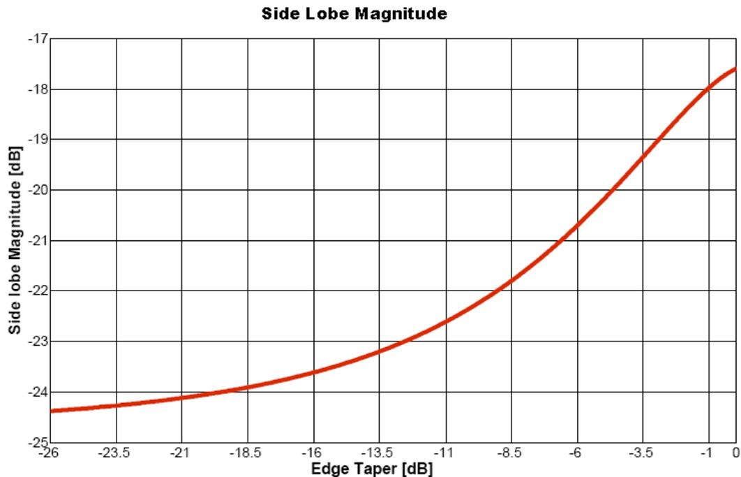
**Fig. 1** – The level of the first sidelobe as a function of the edge taper for quadratic distribution.
