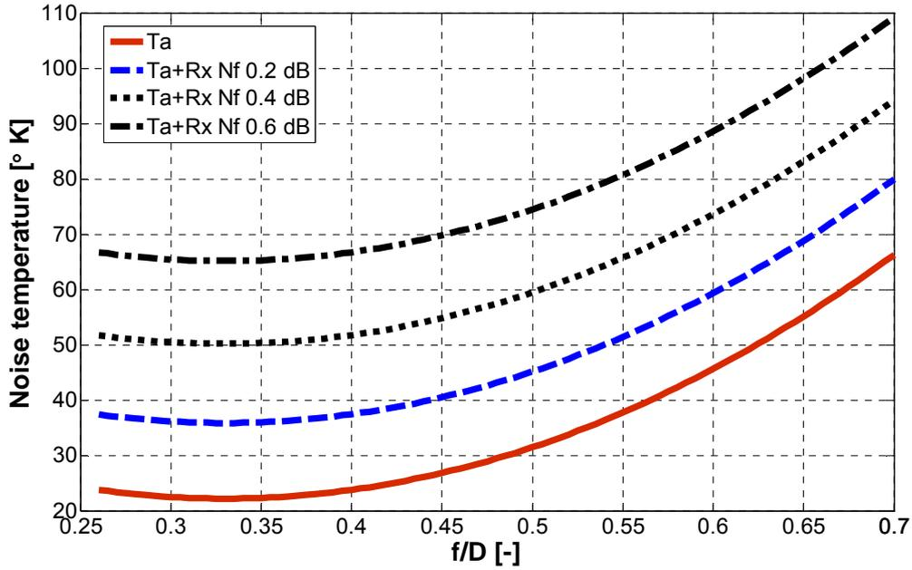
Fig. 8 - Average antenna and system noise temperature
