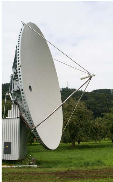
**Fig. 10** - D=10 m Joos (HB9HAL), equipped with dual-mode feed
