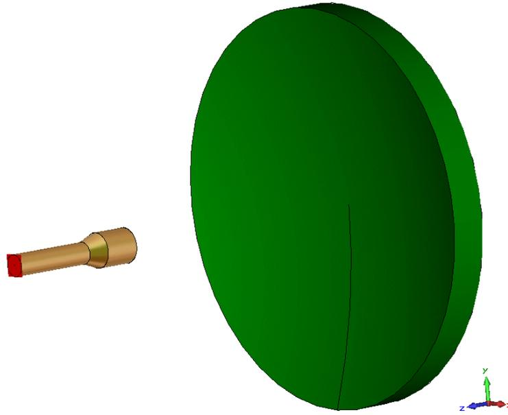
**Fig. 5** – Prime focus dish antenna configuration
