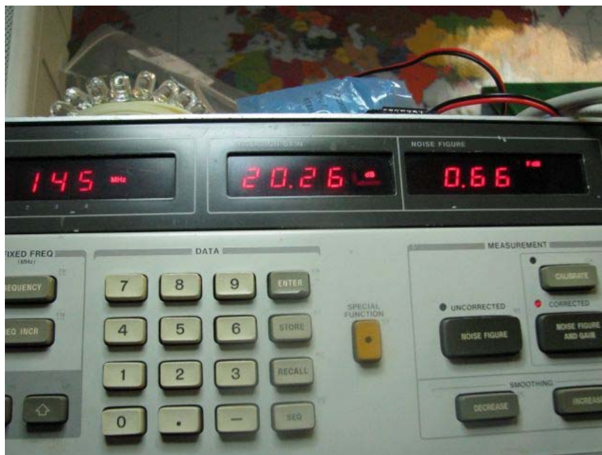
Fig. 25 - Noise figure measurements
