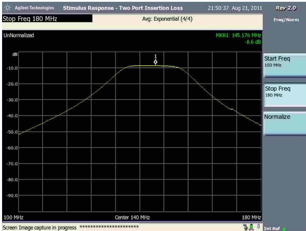
Fig. 6- Two port insertion loss ( S_{21} characteristics) of Temwell TT67381B filter. Insertion loss at 145 MHz is 1 dB.
