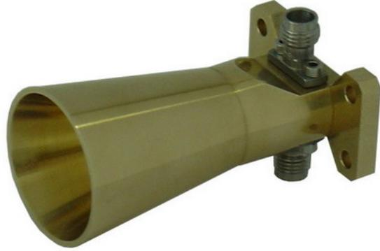
Figure 14: Realized 20 dBi gain septum horn antenna for 47.0 - 48.5 GHz frequency band.
