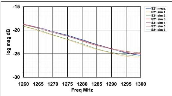
Figure 4 · Comparison of actual measurement data with the simulations of the feed over the frequency span of 1260 MHz to 1300 MHz.
